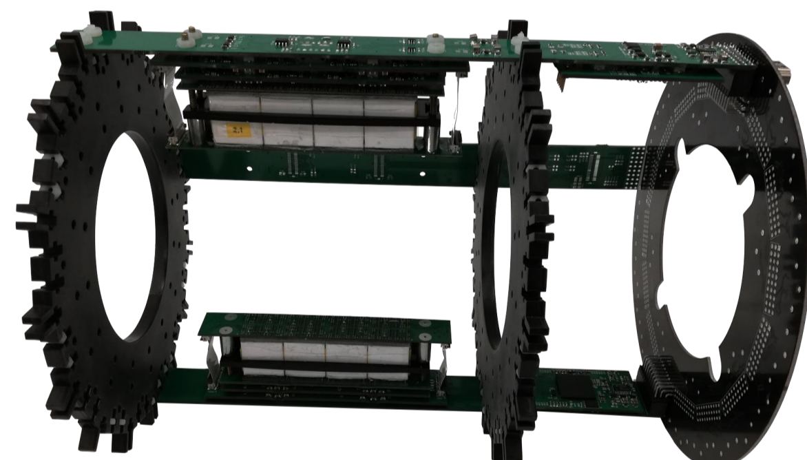
Figure 4: Two modules used to acquire coincidences, mounted on laser cut Delrin rings.
