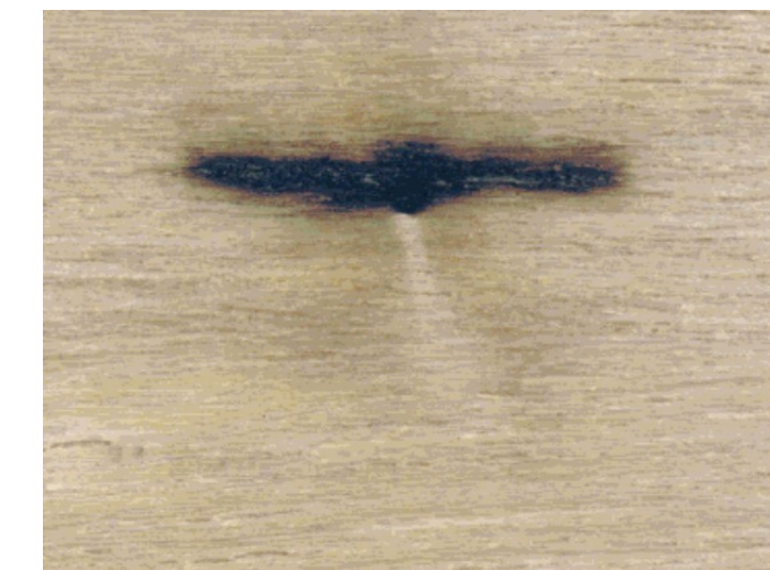
Burn in wood from copper wire at resonant length 3
