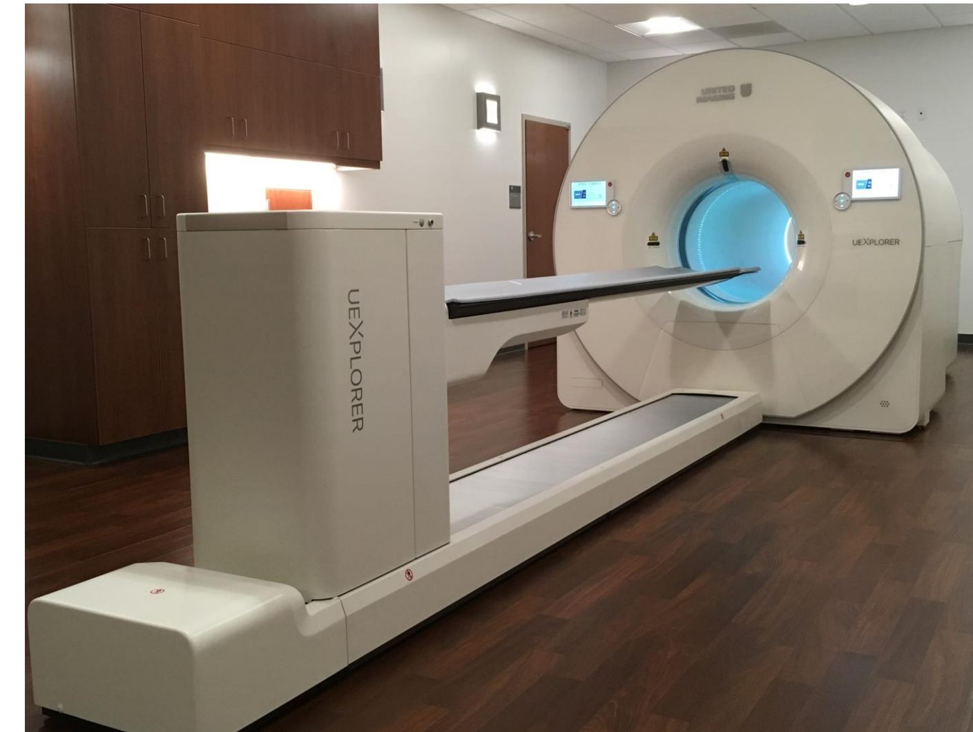
Figure 1 uEXPLORER installed at the EXPLORER molecular imaging center (EMIC) in Sacramento. This is the first clinically operating total-body PET scanner in the US. It has close to 100 B lines of response , which makes data corrections computationally expensive.
